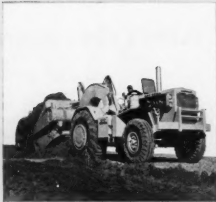
NEW 630 420 HP (335 HP flywheel) . . . 41.5 MPH . . . 630A Tractor-Scraper . . . 28 cu. yd. (21 cu. yd. struck). 630-482C Tractor-Scraper . . . 35 cu. yd. (27 cu. yd. struck).
